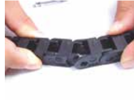
拖链拆分: 然后用力往外扳, 使链节 分离 Chain Separation: Then, switch out the two segments outward with
