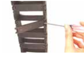
打开横杆: 然后用平头螺丝刀插入横杆右侧的间 隙, 向侧面用力往上撬开横杆的右侧 Open the right side of cover board from the body with screwdriver
