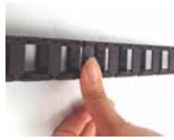
闭合横杆: 旋转横杆, 用手指直接将横杆的 搭扣压入卡槽中 Closed rails: Close the cover board and the body with hand
