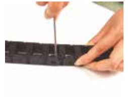
拖链拆分: 在链节与链之间用平头螺 丝刀往外撬, 使销与孔分离 Chain Separation: Separate the one side connect part of two segments by using screwdriver
