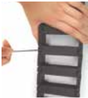
打开横杆: 用平头螺丝刀插入横杆左侧的间隙, 向 侧面用力往上撬开横杆的左侧 Open the left side of cover board from the body with screwdriver
