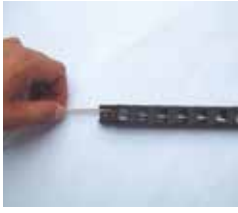
电缆放置: 电缆只能从头往后穿 Cable placement: Put the cables through the chain
