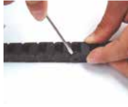
拖链拆分: 在链节与链之间用平头螺 丝刀往外撬, 使销与孔分离 Chain Separation: Separate the segments with screwdriver until the thepunch ate apart from the convex point
